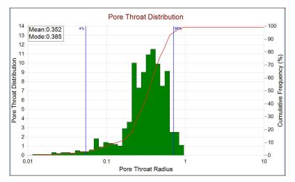
Compute a pore size distribution for each core plug sample and view the distribution of pore throat size in histogram
