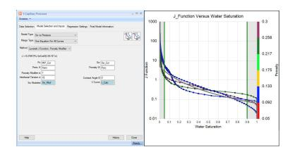
Main module for lab to borehole corrections and Crossplots for quality control of data and models.
