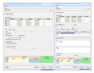
Make pressure corrections in the main module and run calculations using the Capillary Pressure Array Mathpack.
