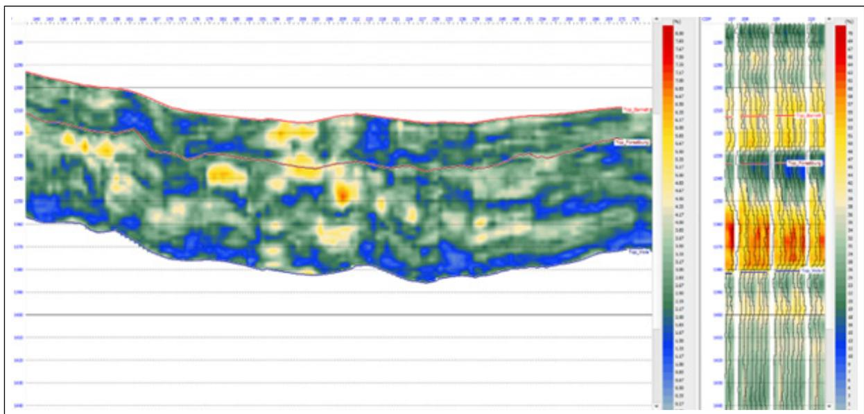
Comparing standard deviation of  $V_{quartz}$  estimation (left) with model prediction variability gathers (right). The highlighted area reflects a larger standard deviation, indicating the high variability in the model's predictions, thus lower confidence.
