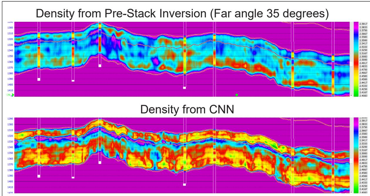
Comparison of Density estimated from pre-stack inversion (top) and from the CNN (bottom). The wells contained in black are the blind wells. CNN estimate has higher detail, matches the well control better and displays higher lateral continuity.
