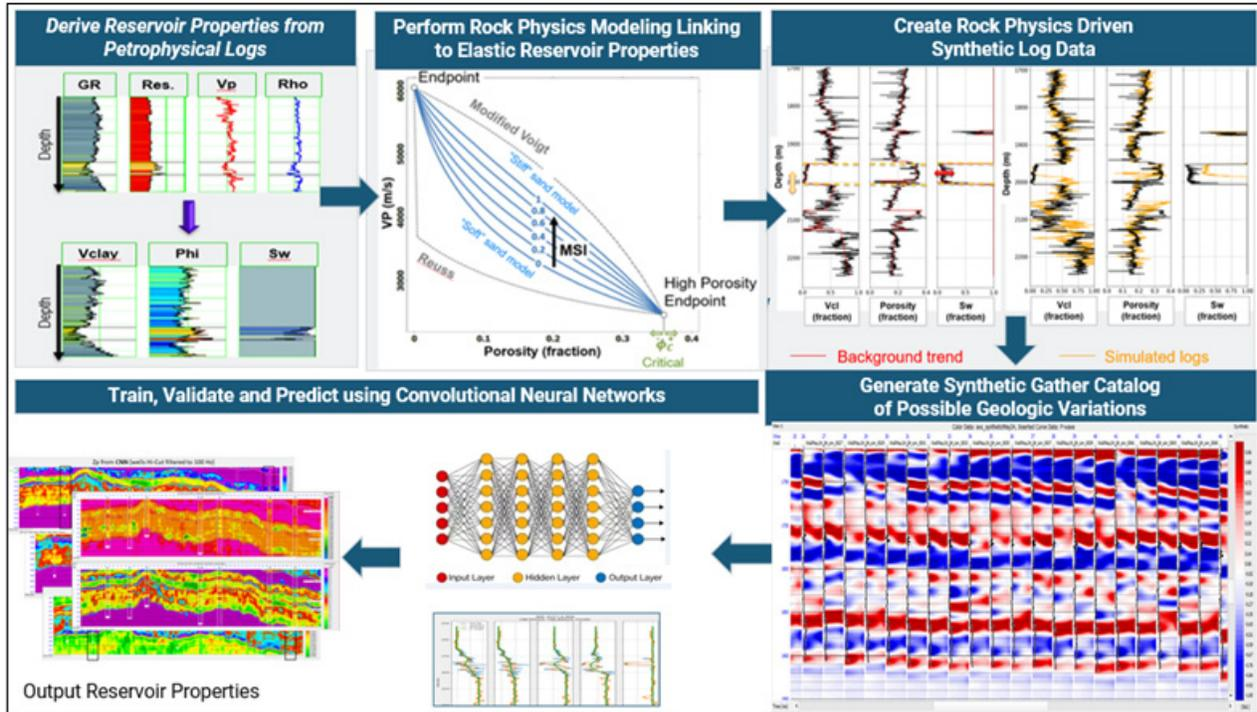
GeoAI workflow: generate synthetic training data based on Rock Physics modelling; create and validate machine learning models; predict reservoir properties as a result.
